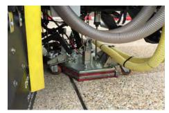
For extra fast cleaning and line removal, the LA2200 can also be fitted with an additional linear cleaning head. Situated under the main chassis, the fixed head provides rapid cleaning and paint removal up to 300mm wide.
